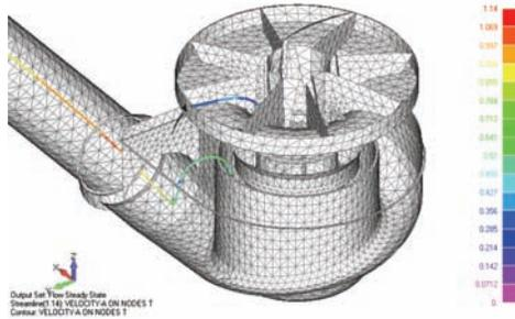
handles disjoint meshes at the fluid/solid boundaries. This unique technology of thermally coupling the disjoint solid and fluid meshes provides a complete solution for simulation of conjugate heat transfer problems.
